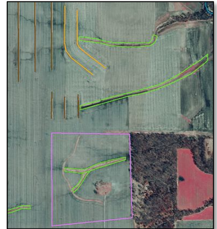
Fayette County, Iowa. 2010 Iowa DNR 0.6-meter spring color infrared aerial imagery showing WASCOS, terraces, contour buffer strip and grassed waterways.
